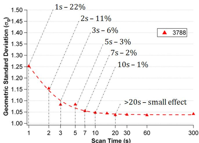
**Figure 4: Geometric standard deviation ( $\sigma_g$ ) of the measured particle size as a function of scan time for SMPS measurements using the Model 3788 Condensation Particle Counter [1].**
