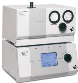
APS configured with optional Aerosol Diluter (Model 3302A) for conditioning high-concentration aerosols.
