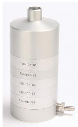
**Figure 2: 130 High-Flow Cascade Impactor**
