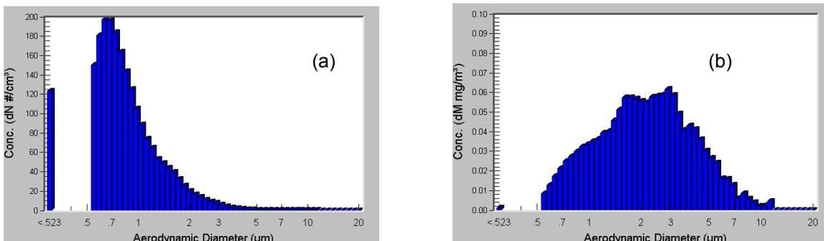
Figure 1. Polydispersed salt (NaCl) aerosol size distributions. (a) APS-measured count-weighted aerodynamic size distribution (b) APS-estimated mass-weighted aerodynamic size distribution using  $\chi = 1$  and  $\rho_p = 2.16 \text{ g cm}^{-3}$ .
