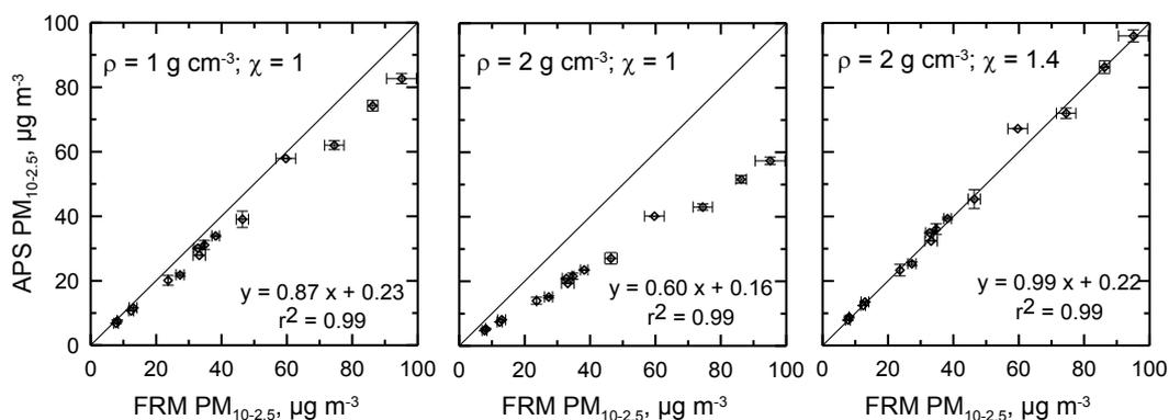
Figure 2. Comparison of PM<sub>10-2.5</sub> estimated with data from APS<sup>TM</sup> spectrometer to that measured with filter-based FRM samplers in Phoenix, AZ.
