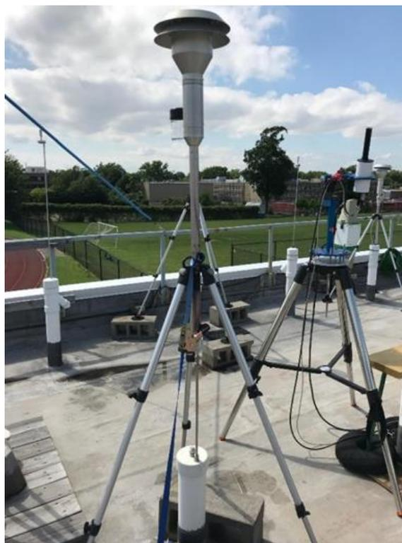
Figure 1: Sampling inlet for QCM-MOUDI™ impactor.
