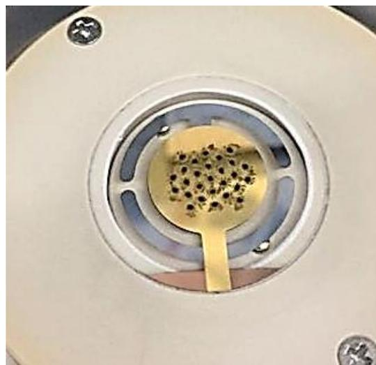
Figure 5: QCM-MOUDI™ impaction plate with collected particles.
