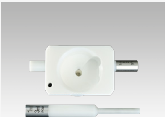
| MEASURING CELL (1 and 3 ml, including piston)
