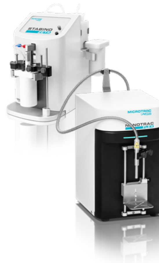
pH Titration of \text{Al}_2\text{O}_3 from pH 4 to 10. The size was measured with the DLS analyzer NANOTRAC FLEX to determine the conglomeration point
