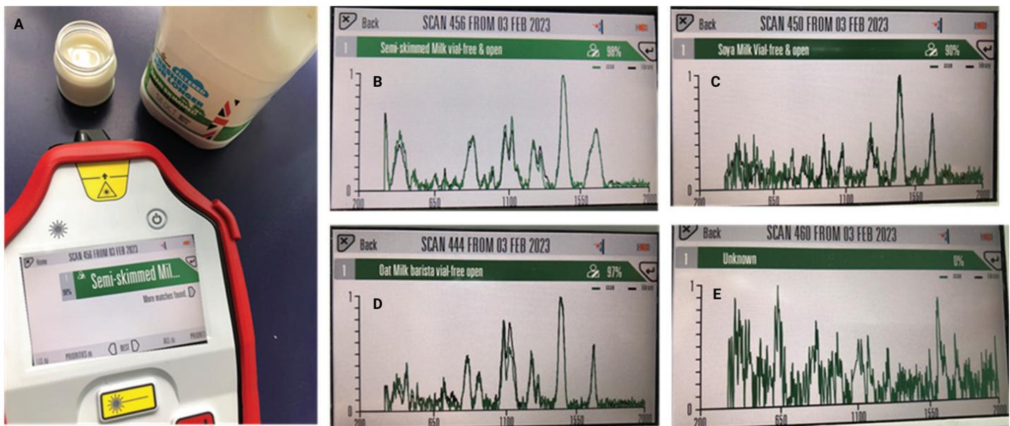
**Figure 4.** (A) Agilent Resolve Raman handheld analyzer and small plastic container of semi-skimmed milk. (B) Scan of semi-skimmed milk with a match quality of 98%. (C) Scan of soy milk with a match quality of 90%. (D) Scan of oat milk with a match quality of 97%. (E) Scan of water (no match 0%).
