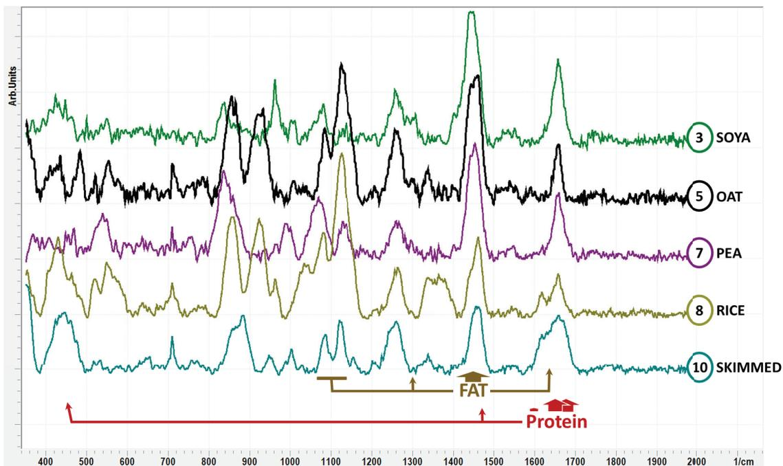
**Figure 5.** Raman spectra of selected milks (soy, oat, pea, rice, and skimmed dairy milk), highlighting the peak band assignments for fat and protein. The large arrows represent a major contributor, while the smaller arrows indicate a less significant contribution. The flat bars represent a variable contribution.
