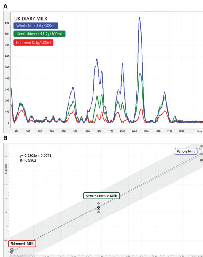
**Figure 7.** (A) Raman spectra collected in barrier-free surface scan mode of three common UK grades of milk: skimmed (red, 0.1 g/100 mL fat), semi-skimmed (green, 1.7 g/100 mL fat), and whole milk (blue, 3.6 g/100 mL fat). (B) Actual versus predicted MVA-PLS1 model for the milk fat for the three common classes of dairy milk. The training calibration spectra are shown by the black markers and the validation spectra are shown by the blue diamonds.
