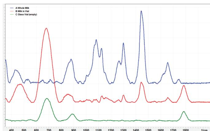
**Figure 2.** Stacked Raman Resolve spectra. Green: empty clear glass vial; red: whole milk in a glass vial (vial mode); blue: spectrum that was collected directly from the whole milk sample in surface scan (barrier-free) mode.
