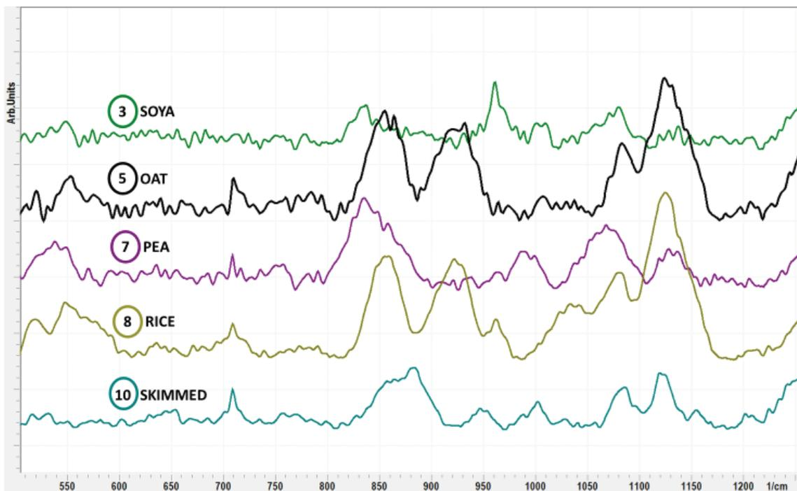
**Figure 6.** The main carbohydrate region of Raman spectra ( $500$  to  $1,200\text{ cm}^{-1}$ ) for selected plant and dairy milks.
